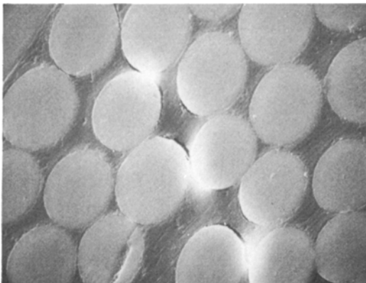
Figure 13 Fibre debonds at \sim 0.5\% strain ( \times 1290 ).
